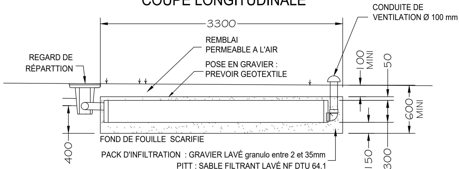
LE PACK D'INFILTRATION EST GARANTIE POUR UNE PERMÉABILITÉ MINIMUM DE 10mm/H AU NIVEAU DU FOND DE FOUILLE; SOIT 40CM SOUS FIL D'EAU D'ENTRÉE DANS LE REGARD DE REPARTITION. IL EST IMPÉRATIF DE S'ASSURER QUE LA PERMÉABILITÉ SOIT TOUJOURS DE 10mm/H AU MINIMUM MALGRÉ LA PROFONDEUR VARIABLE SELON CHAQUE CHANTIER. EN CAS DE DOUTE, FAIRE RECONFIRMER LA PERMÉABILITÉ PAR LE BUREAU D'ETUDES.
